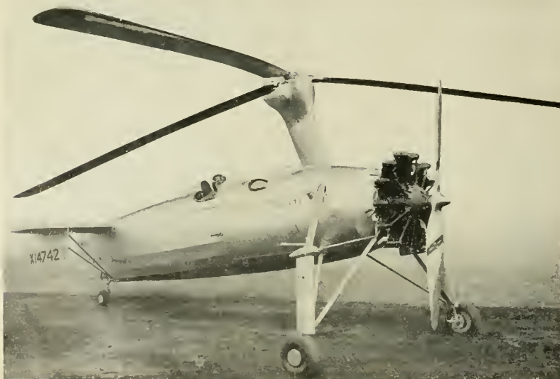
Kellett's open-cockpit version of the wingless autogiro with 225 h.p. Jacobs engine
